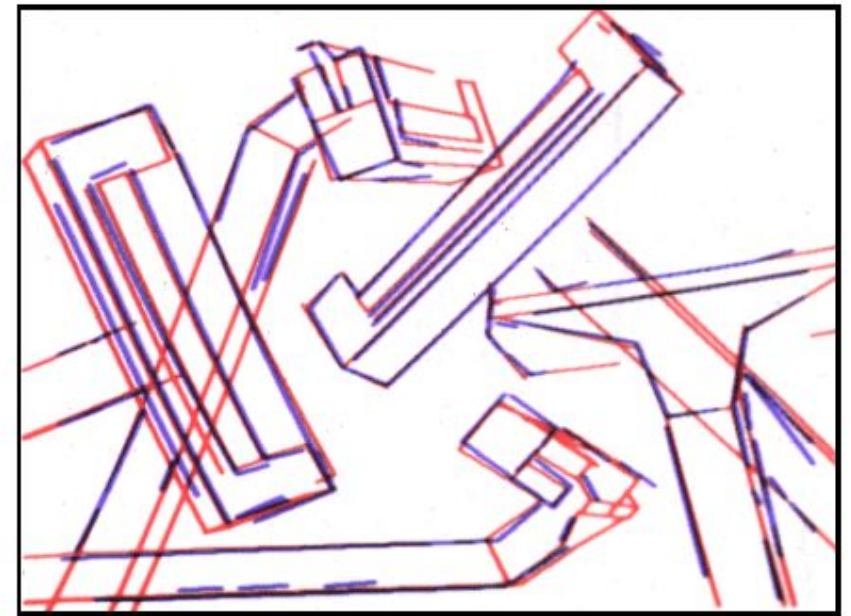
Figure 14: Successful matches between sets of image segments and particular view points of the model.
